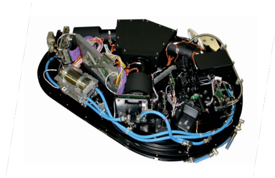
Design 1: Airborne Prism Experiment (APEX) Imaging Spectrometer
